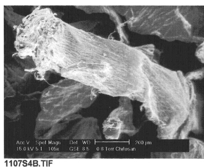
FIGURE 6 SEM of chitosan.
